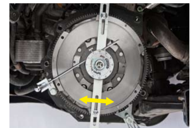
Measuring freeplay angle
